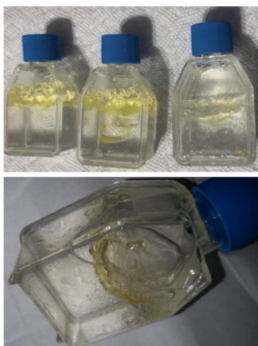
Figure 2: Production of lipoprotein hydrogel from microculture at water-oil interface
